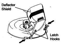
**ACAUTION:** Do not remove discharge guard from mower. Raise and hold guard when attaching mulcher plate and allow it to rest on plate while in operation.
