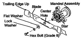
**IMPORTANT:** Blade bolt is grade 8 heat treated.
